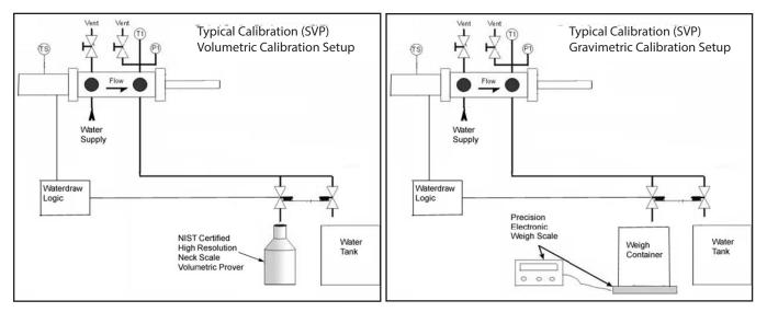
Preparation of the Prover in both cases is identical. Conducting the calibration runs is nearly identical in both cases. Gathering and recording the required data to calculate the base volumes of displacement and tank Provers is nearly identical for the volumetric method and gravimetric methods. Calculations are identical for correcting the Prover volume for pressure and temperature in both techniques.
