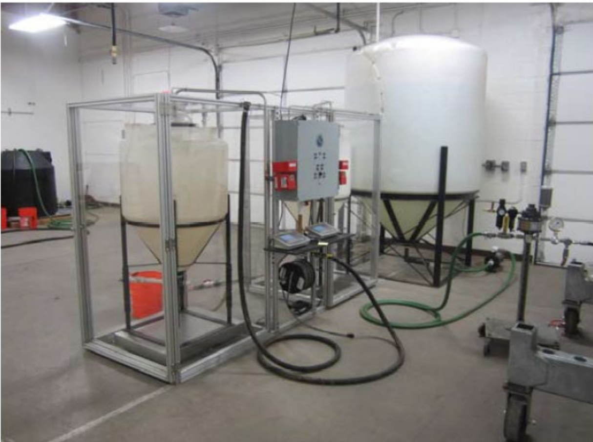
Figure 4: ISO 17025 Certified Gravimetric Water Draw Test Stand – Flow MD – Phoenix, AZ
