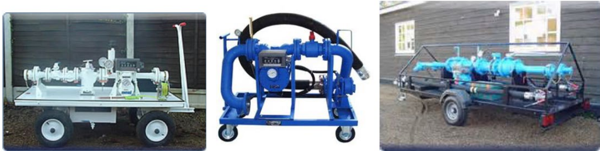
Figure 5: Master Meter Cart and Trailer Designs
